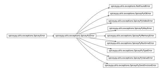
Spice defines hundreds of errors in the format "SPICE(ERROR\_NAME)" which are also included in SpiceyPy by a slightly different naming convention, where a Spice error "SPICE(QUERYFAILURE)" will correspond to the SpiceyPy exception <code>spiceypy.utils.exceptions.SpiceQUERYFAILURE</code>.
